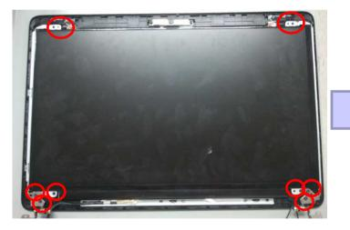
Loose LCD & Hinge screw, take off LCD , hinge and panel.
